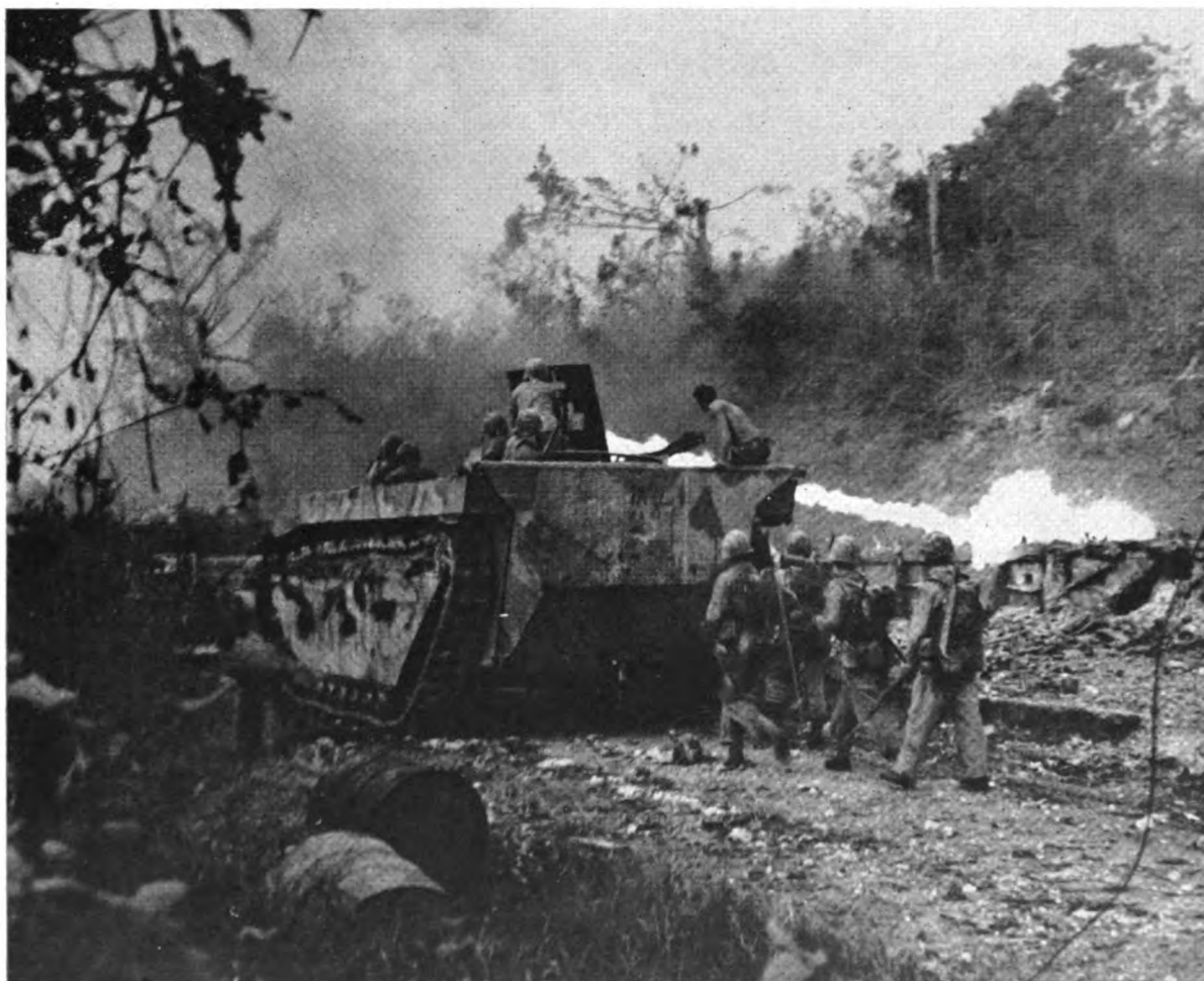
LONG RANGE FLAME-THROWERS were first used at Peleliu. LVT mount was thereafter replaced by tank.
