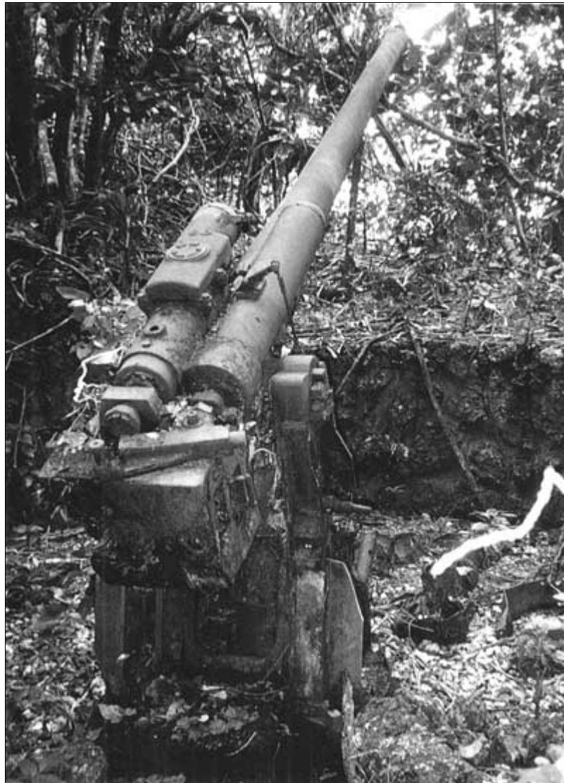
Possibly one of the best preserved specimens of its kind in the Pacific, this Model 10 120mm dual-purpose antiaircraft and coastal defense gun is on the western shore of Ngesebus. The gun rests on its skid plate and was sited in a natural position. Caption and photo Dr. Phillip D. Orr
